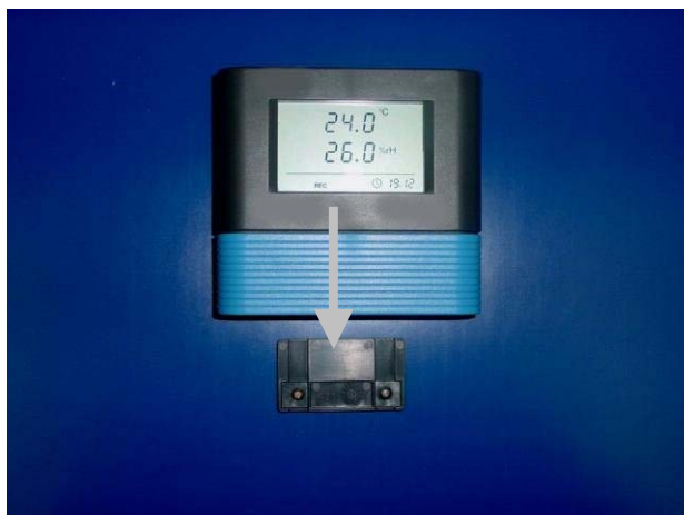
Fig.: Hanging in the datalogger on the angle
