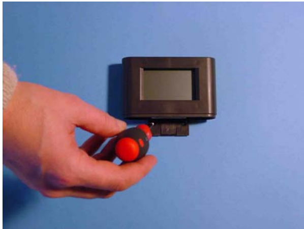
Figure: mounting the datalogger
