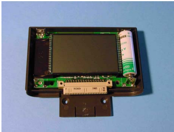
Figure: changing the battery
