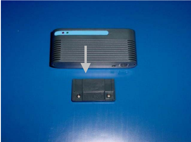
Fig.: Mounting of a datalogger without display
