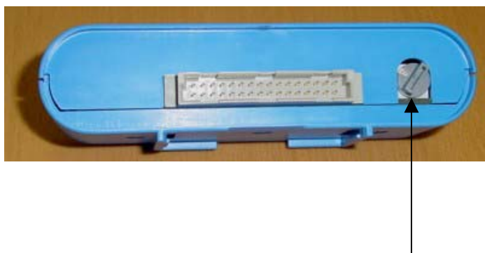
Rotary switch to set up TC
