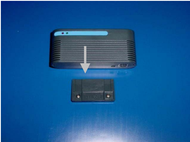
Fig.: Mounting of a datalogger without display
