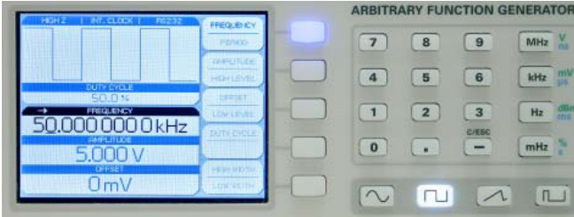
Fig. 4.3: Front view including display of the settings
