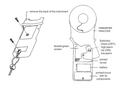
According to the type of alarm selected, crossing of the alarm threshold will be indicated by the appearance of an or and a continuous beep at high or low frequency.
