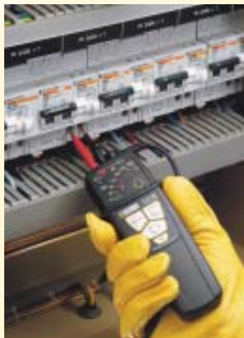
Used together, the C.A 751 + C.A 760 create a resistive phase-earth link for safely testing a 30 mA circuit breaker at 230 V AC.
