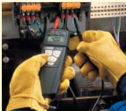
Phase rotation direction is defined by a TT, TN, or IT neutral system due to an innovative 2-wire method. This test operates on generator sets.
