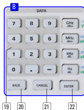
Fig. 4.1: Section B with numerical keyboard, unit and command keys
