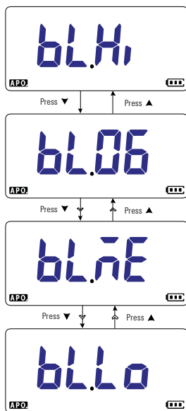
Figure 4-7 Changing the LCD backlight intensity
