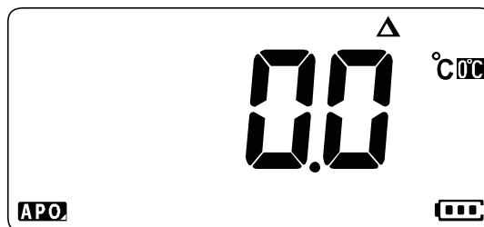
Figure 2-21 Temperature measurement without ambient compensation
