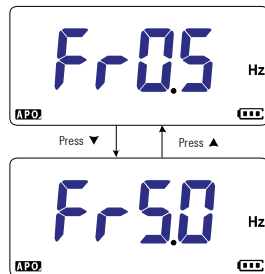
Figure 4-10 Changing the minimum measurable frequency
