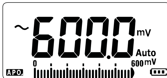
Figure 2-1 AC voltage display
