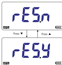
Figure 4-13 Resetting the Setup items
