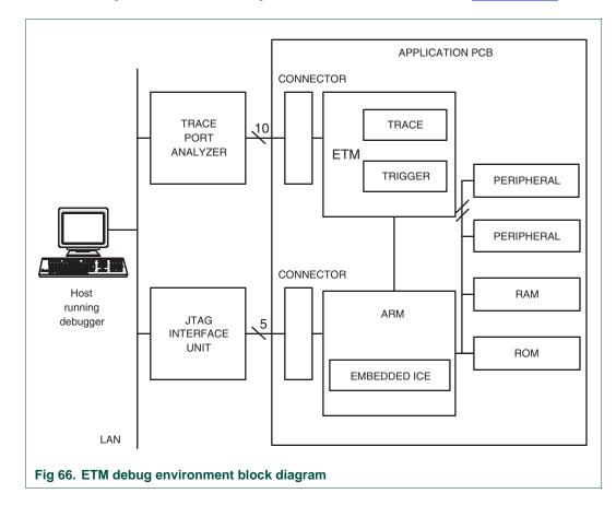
The block diagram of the ETM debug environment is shown below in Figure 21–66.
