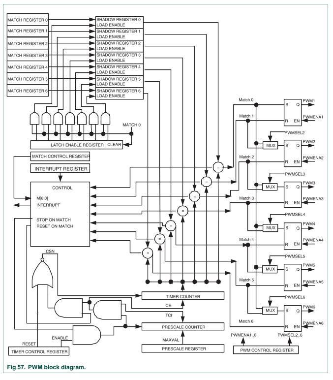
A sample of how PWM values relate to waveform outputs is shown in Figure 15–58. PWM output logic is shown in Figure 15–57 that allows selection of either single or double edge controlled PWM outputs via the multiplexers controlled by the PWMSELn bits. The match register selections for various PWM outputs is shown in Table 15–186. This
