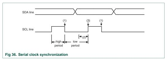
A slave may stretch the space duration to slow down the bus master. The space duration may also be stretched for handshaking purposes. This can be done after each bit or after a complete byte transfer. the I<sup>2</sup>C block will stretch the SCL space duration after a byte has been transmitted or received and the acknowledge bit has been transferred. The serial interrupt flag (SI) is set, and the stretching continues until the serial interrupt flag is cleared.
