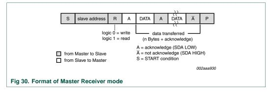
After a repeated START condition, I<sup>2</sup>C may switch to the master transmitter mode.
