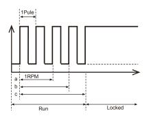
The relationship between rpm & output pules signal from 3rd wire are as follows:
