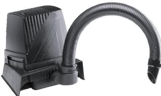
The BVX-100 can also be used with bench-mounted arms normally used with multi-user systems. Remove the arm and nozzle from the arm adaptor assembly. Insert the 50mm hose, supplied with the arm, into the arm adaptor assy.
