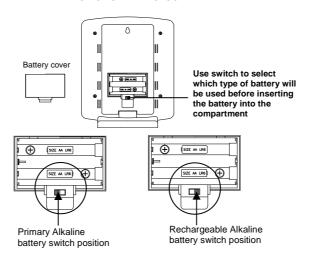
Note: For best performance, batteries should be replaced at least once every 2 years to maintain the best running accuracy. Ensure that the batteries used are new and the correct size.
