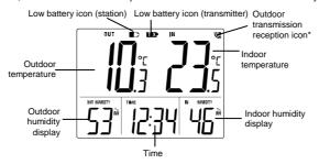
\* When the signal from the transmitter is successfully received by the Solar Station, this icon will be switched on. (If not successful, the icon will not be shown on the LCD). User can therefore easily see whether the last reception was successful ("ON" icon) or not ("OFF" icon). On the other hand, the short blinking of the icon shows that a reception is being done at that time.
